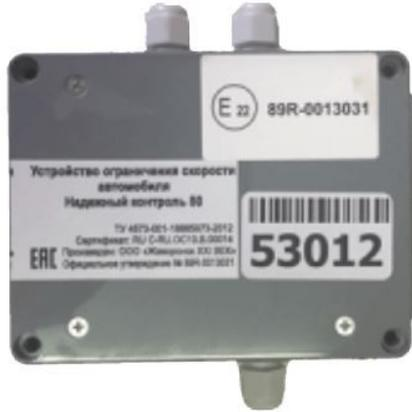
PICTURE 1. SPEED LIMITATION DEVICE (SLD) TYPE NK-80.
